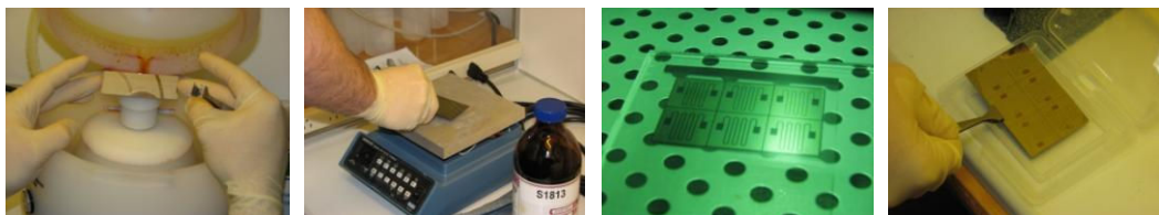
Figure 7. Fabrication of an RTD using photolithography.
