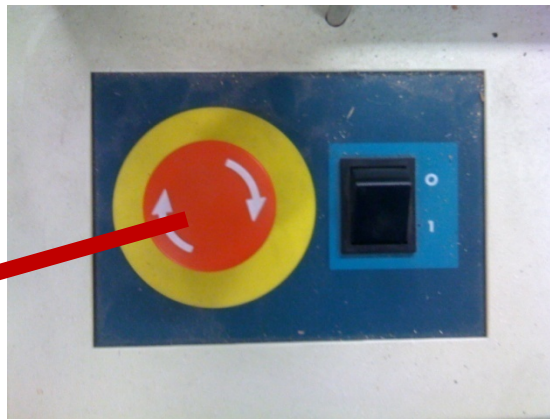
Figure 2. E-Stop and main power switch.
