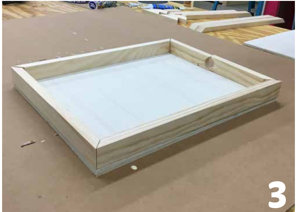
Arrange the 1x2 frame components on top of the plywood base to begin the "Vacuum Box"
