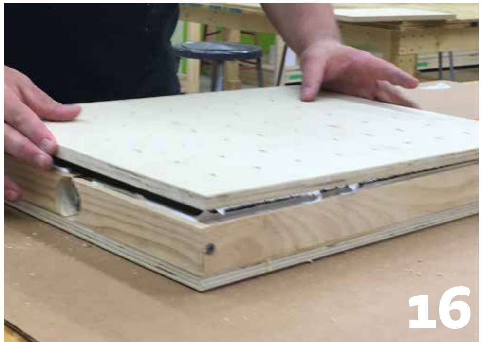
Place the drilled top onto the caulked frame to complete the Vacuum Box.
