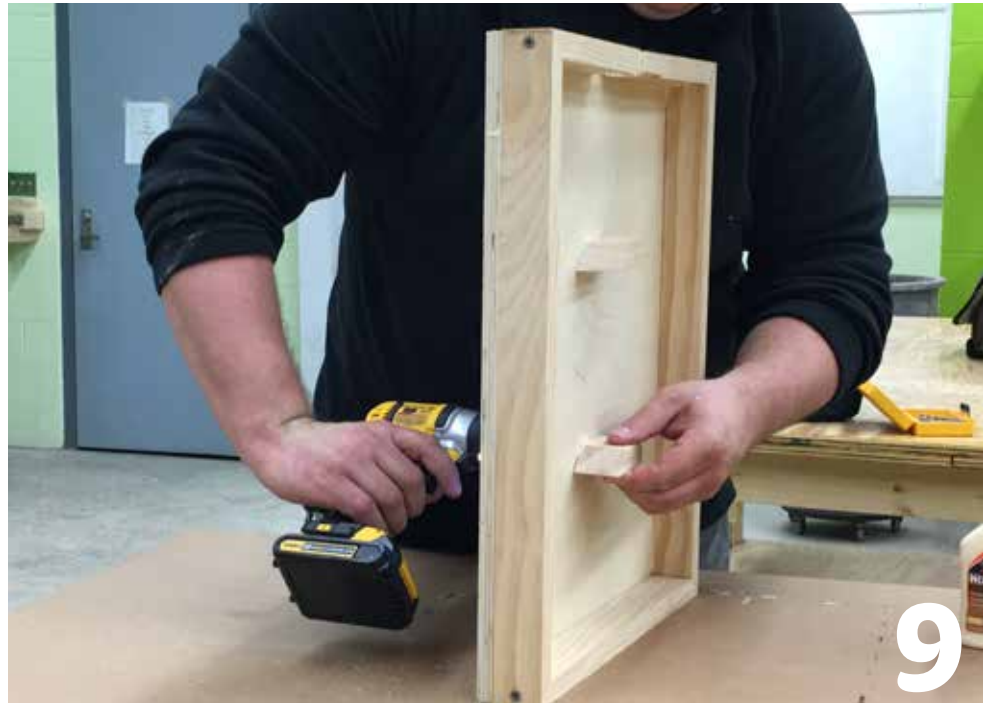
Holding the block ready, place a screw into it through pilot hole drilled earlier. Ensure that its held down tight to the base.
