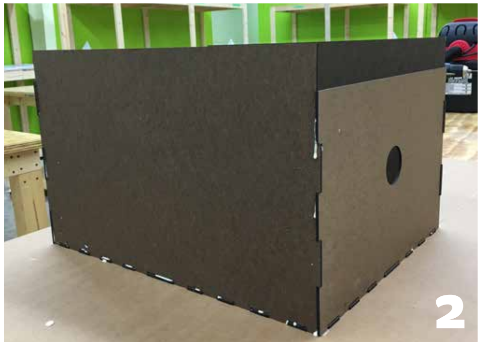
Assemble the "Warming Box". Tape can be used to hold the box together temporarily while the glue dries.
