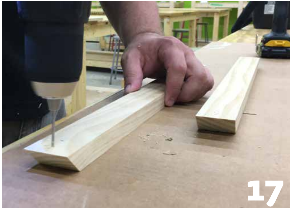
Time to build the sheet frame: Start by drilling pilot holes in the mitered ends of the other 1x2 frame parts.
