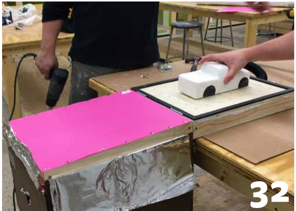
Place the object to be formed in plastic on the drilled surface of the vacuum box.
