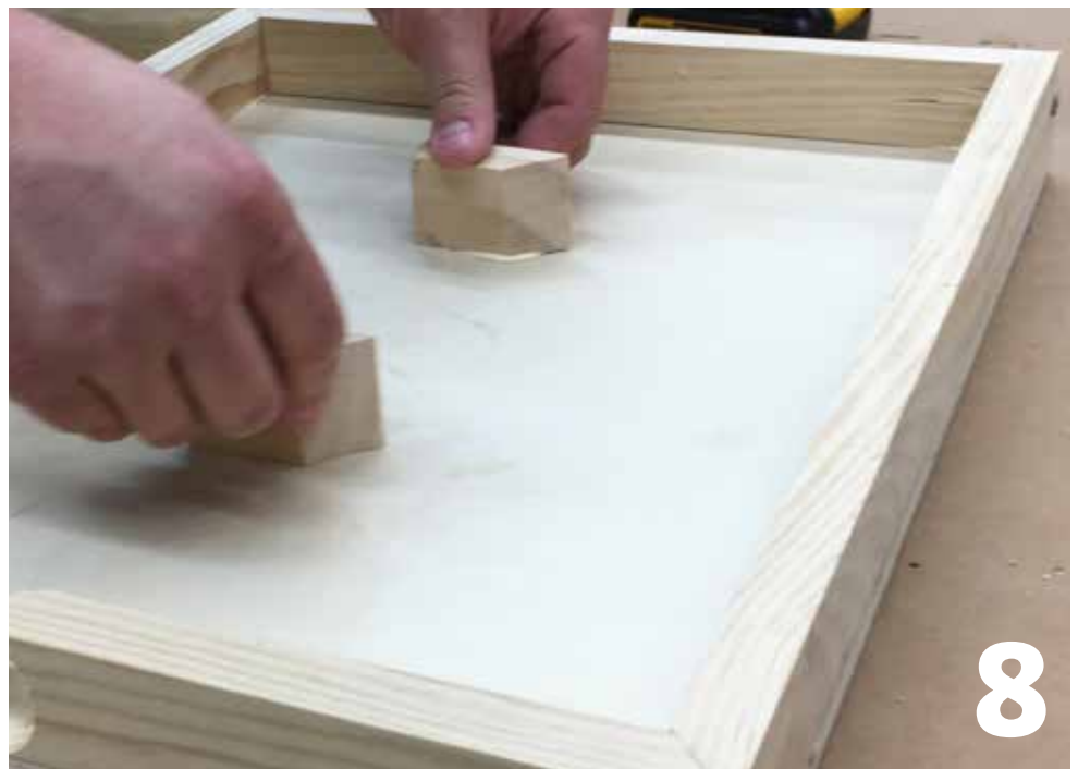
Glue blocks over holes inside the frame.
