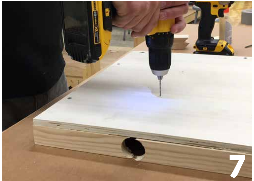
Place 2 more holes near the center of the frame for attaching block supports.
