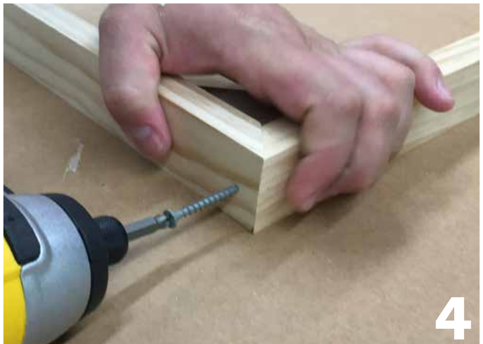
Drill an 1/8" pilot hole in the side of the frame, then use a screw to attach the frame edges in a tight 90° corner. Repeat these steps for all four corners.
