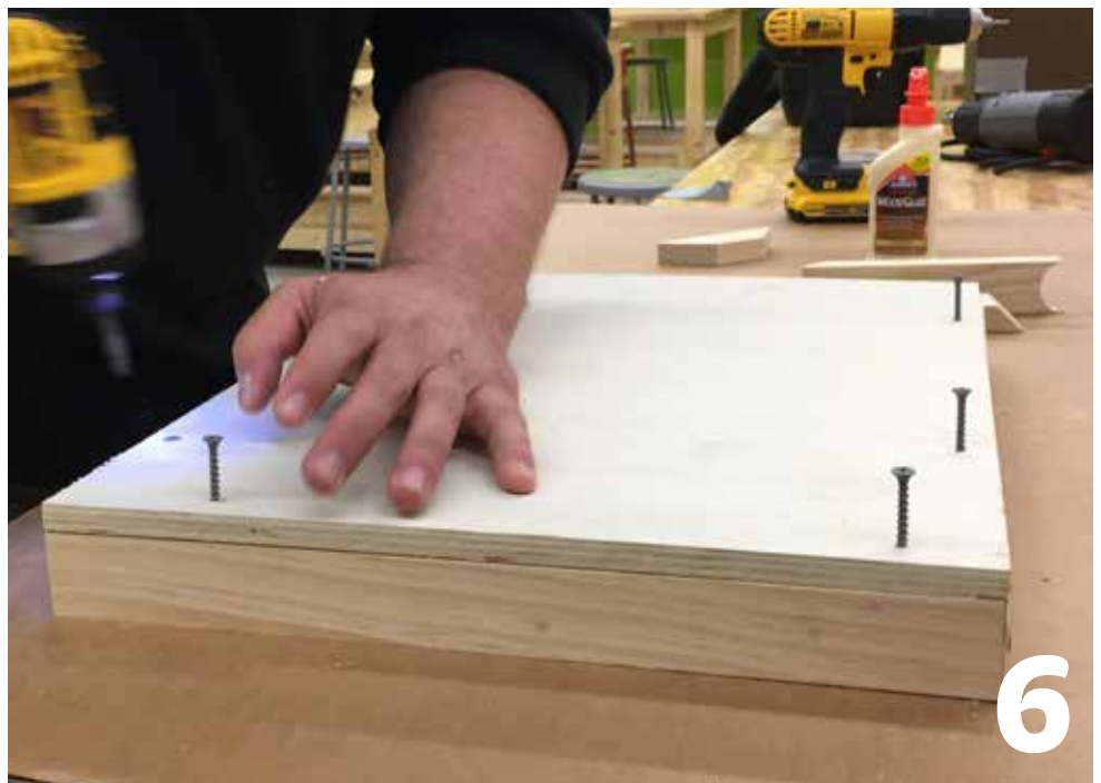
Insert screws into the pilot holes and fasten the base to your assembled 1x2 frame. Make sure the seams are tight.
