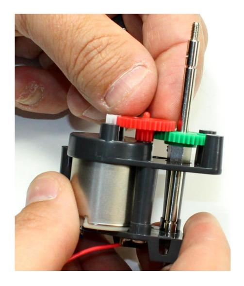
install red gear, contacting motor pinion gear and the green axle gear
