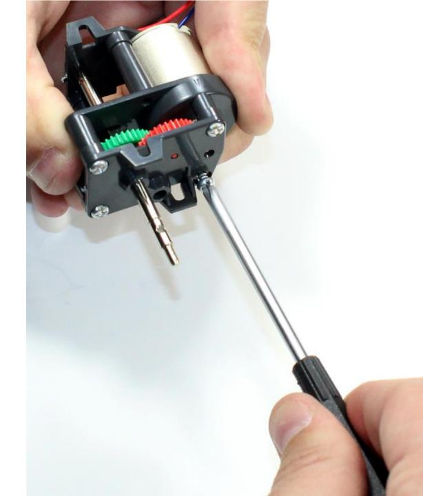
install roll pin until it is centered on axle shaft
