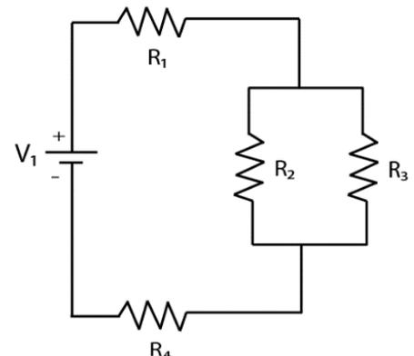
4. Find the equivalent resistance for the given circuit.  $R_{eq} = 684.25\Omega$
