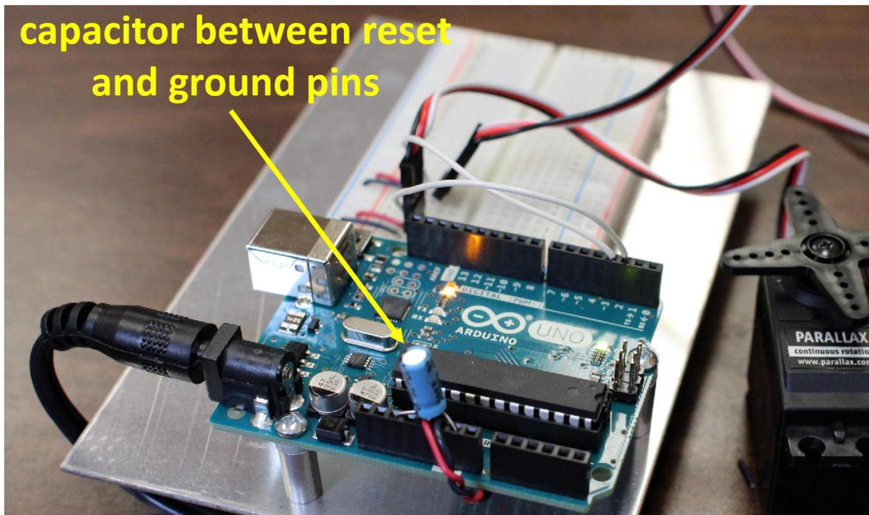
To illustrate the difference that a capacitor makes in the voltage at the reset pin, we can use a device called an oscilloscope to plot voltage versus time. See the photo below that shows the voltage at the reset pin when no capacitor is installed. Notice that the voltage drops from 5V to almost 3V (a 2V drop) when no capacitor is present. For the settings on the oscilloscope shown, the divisions on the y-axis (voltage) are 1V apart, and the divisions on the x-axis (time) are 500ms apart.
