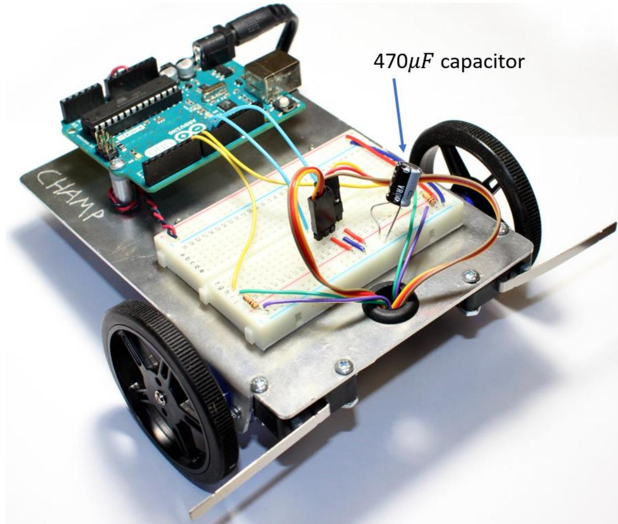
This larger capacitor would work like the 10 $\mu$ F capacitor described above, but with much more capacity to smooth out sudden fluctuations in voltage. Also, putting the capacitor nearer the source of the sudden energy demands (associated with a servo starting up or changing direction) would help shield the Arduino from the voltage fluctuations altogether. See the link below for the writeup from adafruit.
