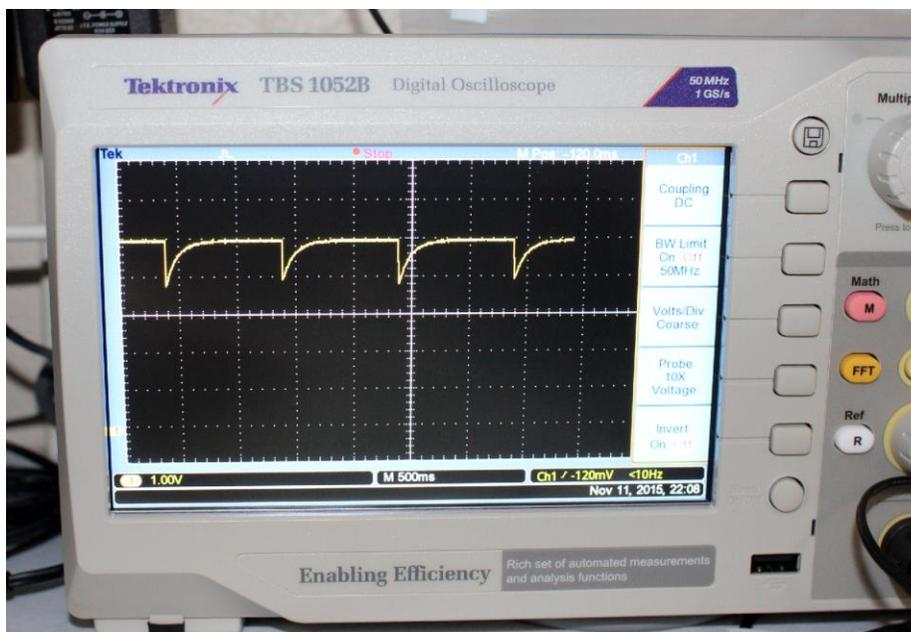
When a capacitor is used, notice how the voltage builds slowly back up to 5V when the servos change direction. This is because the capacitor is recharging during this time. If a larger capacitor such as a 1000 $\mu$ F were to be used, the voltage drop would be smaller when the servos changed direction; however, adding a capacitor this large would delay the start of a program since it would take a while for the capacitor to charge up before the program could start running for the first time.
