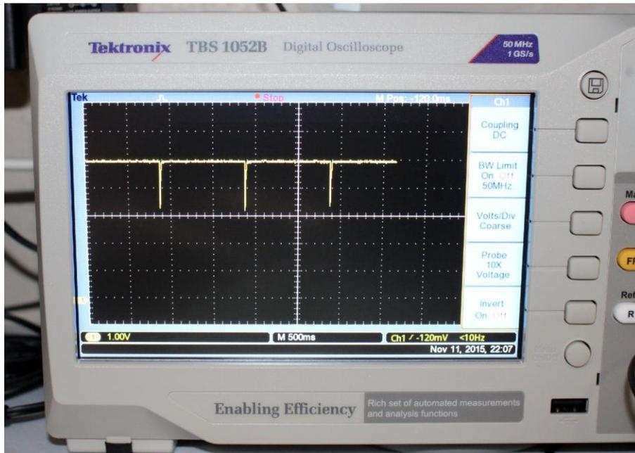
The voltage drop at the reset pin is about 1V when a 10 $\mu$ F capacitor is used:
