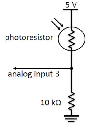
6. Refer to the photoresistor circuit shown. If the analogRead(3) function is used to determine the voltage at analog input 3 and the value returned is "VAL" (given below), the voltage would be closest to:
