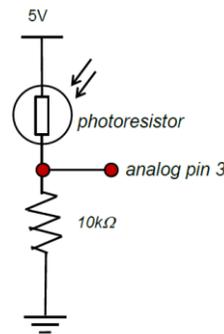
3. When the photoresistor in the circuit diagram below has a resistance of  $20\text{ k}\Omega$ , the integer value returned by the `analogRead(3)` function will be closest to:
