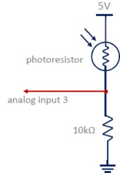
2. The photoresistor circuit used in class is attached to analog input 3 to “measure” the light level. If the light level is such that the resistance of the photoresistor is  $2,000\ \Omega$ , then the Serial Monitor will show that “val” is closest to . . .
