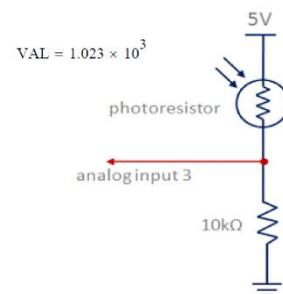
9. Assume the voltage at analog input 3 is as given below. The resistance value of the photoresistor is closest to:
