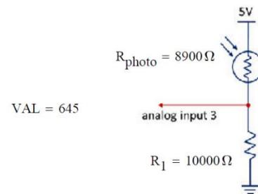
7. Refer to the above photoresistor circuit shown. Assume the voltage at analog input 3 is given below. The resistance value of the photoresistor in this state is closest to:
