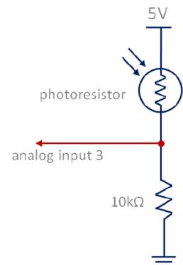
4. Assuming the resistance of the photoresistor in the problem below is  $100\Omega$ , then the power dissipated at the photoresistor is closest to:
