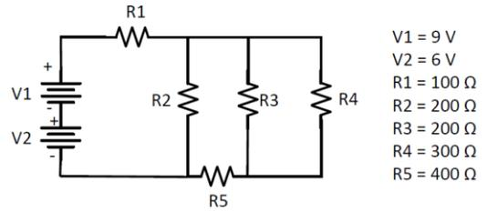
21. The equivalent resistance of all the resistors in the circuit shown below is closest to...
