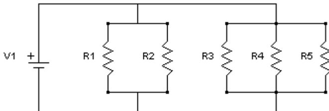
17. For the circuit below (where  $V_1 = 12V$ ,  $VR_1 = 3.02V$ ,  $VR_2 = 1.19V$ ,  $VR_3 = 0.38V$ ,  $VR_4 = 4.67V$ , and  $VR_6 = 2.09V$ ), the voltage drop across  $R_5$  is closest to ...
