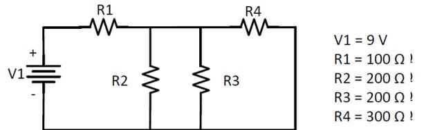
19. The current through  $R_3$  for the circuit shown below is closest to...
