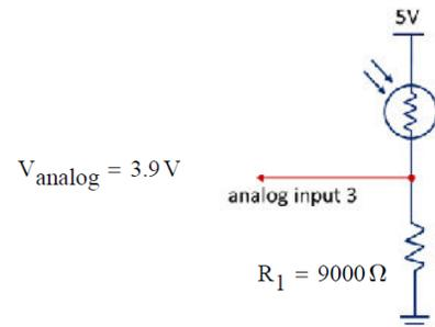
8. If the analogRead(3) function is used to determine the voltage at analog input 3, and the value returned is "VAL" (given below), the voltage would be closest to:
