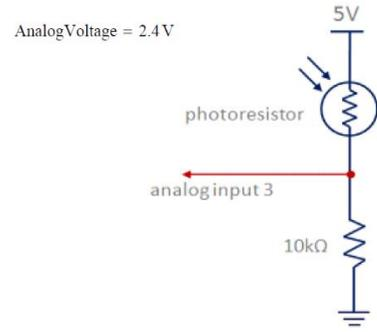
10. The photoresistor circuit used in class is attached to analog input 3 to “measure” the light level. If the light level is such that the resistance of the photoresistor is 3,000 $\Omega$ , then the Serial Monitor will show that “val” is closest to . . .
