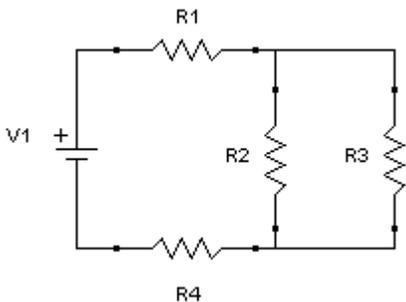
15. For the circuit below (where  $V_1 = 24V$ ,  $R_1 = 100\Omega$ ,  $R_2 = 200\Omega$  and  $R_3 = 300\Omega$ ) the power dissipated by  $R_2$  is closest to ...
