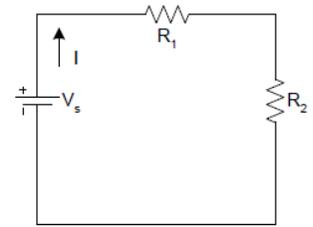
30. For this diagram,  $V_s = 20V$ ,  $R_1 = 50\Omega$ , and  $I = 0.2A$ . The value of  $R_2$  is most nearly:
