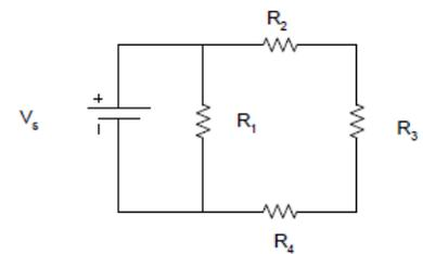
29. For this diagram,  $V_s = 20V$ ,  $R_1 = 50\Omega$ , and  $I = 0.2A$ . The power generated by the voltage source is most nearly:
