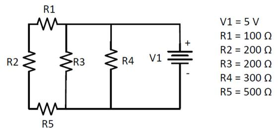
20. The power dissipated by R2 for the circuit shown below is closest to...
