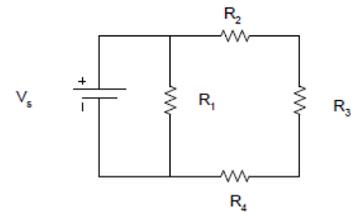
28. If  $R_{eq}$  for the circuit is  $100\Omega$  and  $V_s$  is  $20V$ , then the power generated by the voltage source is most nearly:
