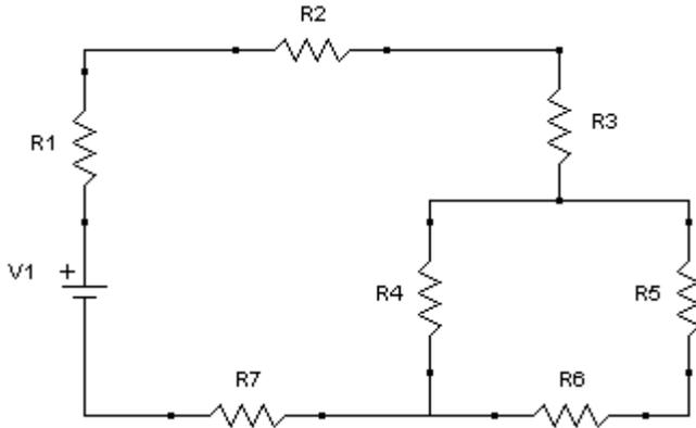
18. The voltage drop across  $R_1$  for the circuit shown below is closest to...
