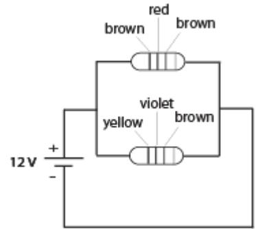
13. The equivalent resistance of the following circuit is closest to . . .
