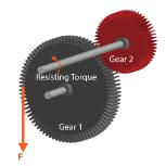
4. The max speed for the servo shown is 130RPM when connected to 6V. Assume that the gearbox on your servo is able to output a torque of 1.5 kg-cm while turning at this speed. Using the number of teeth on each gear provided in the table, determine the torque and rotational speed of the *output shaft on the DC motor*. 30515.086 RPM and 0.0627 N-cm
