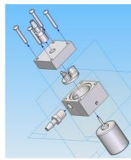
Figure 4. Centrifugal pump and its solid model.
