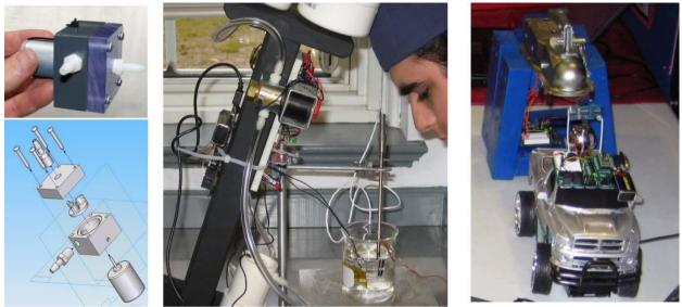
Figure 2 – Example projects, including the centrifugal pump (left), the fishtank (center), and a smart trailer hitch which provides an example of an innovative product (right)
