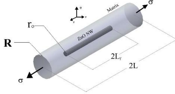
**Figure 1.** RVE of a ZnO NW with length of  $2L_f$ , embedded in a matrix with length of  $2L$ . The composite is subjected to the overall stress of  $\sigma$  along the cylindrical axis.  $R$  is the outer radius of the RVE and  $r_o$  is the radius of the ZnO NW. Reprinted with permission from J. Appl. Phys. 108(11), 114303 (2010). Copyright 2010 American Institute of Physics.[19]
