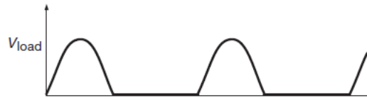
Figure 1.57. Half-wave output voltage (unfiltered).
