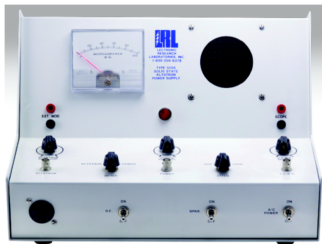
Figure 6: The Klystron power supply, the signal amplifier and the DC current meter included in the unit 510A
