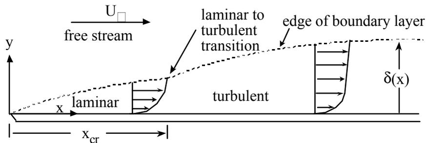
Fig. 7.1 Schematic of boundary layer flow over a flat plate
