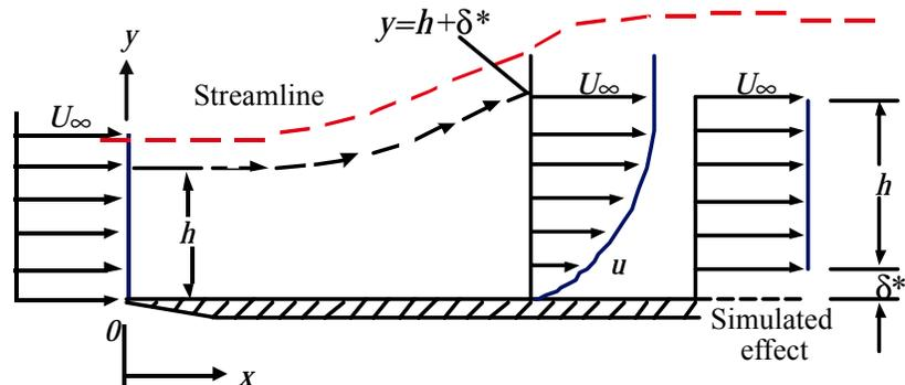
A viscous boundary layer is created when the flow comes in contact with the solid surface.
