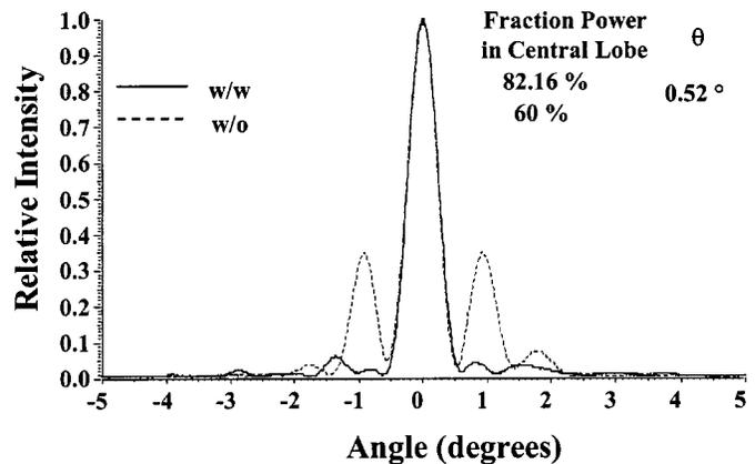
Fig. 5. Far-field distribution of the taper amplifier with and without the grating for  $I = 3$  A.
