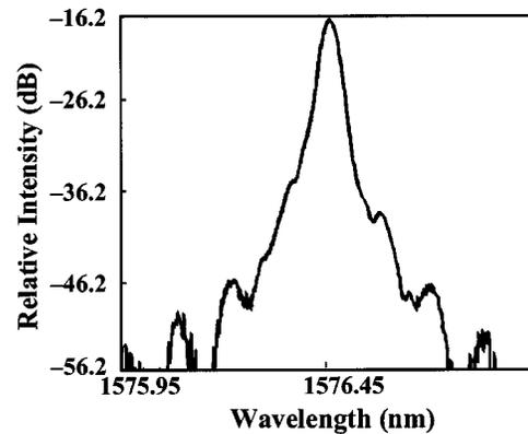
Fig. 4. Wavelength spectrum for the DBR tapered laser at 3 A. The spectrometer resolution is 0.05 nm.
