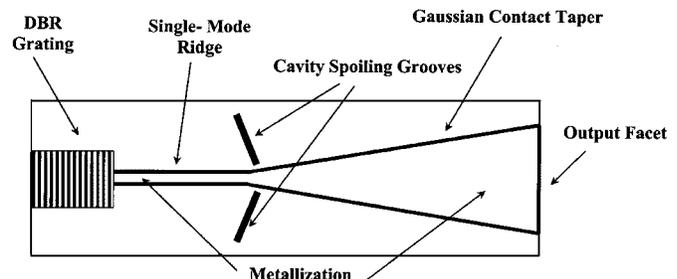
Fig. 2. Schematic illustration of DBR tapered laser.
