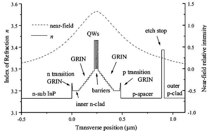
Fig. 1. The vertical index of refraction and calculated vertical mode intensity profiles in epitaxial structure.
