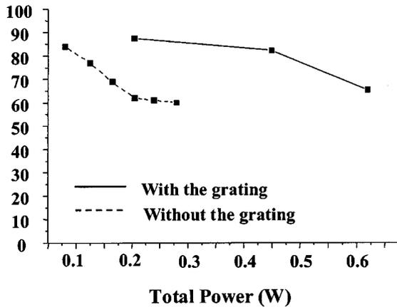
Fig. 6. Central lobe power versus total optical power for tapered lasers with and without a DBR grating.
