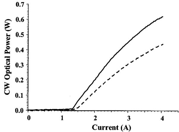
Fig. 3.  $L$ - $I$  CW characteristics for tapered lasers with (solid curve) and without (dashed curve) the DBR grating.
