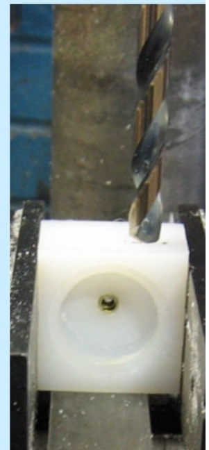
Figure 7 – Pressing in O-Ring Retainer (Top) and Preparing to Drill Water Exit (Bottom)
